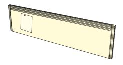
400mm high (1114mm overall from floor), 30mm thick fabric panel with three sided aluminium rail surround trim (top and sides). 20mm gap between screen and MFC top for cable access on double row benches. Add screen frame colour code (eg /W) then add /A (or other) to the end of the code to denote band choice (page 22).
