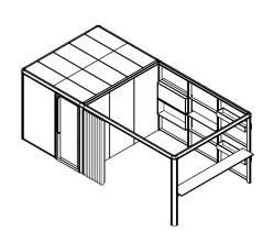
Hush Hideout 2180x1140mm with glazed with door, three fabric panels, vertical power rail & wall mounted power outlets and worksurface. Ecophon acoustic ceiling kit incorporating air flow circulation system and LED lighting controlled by PIR motion detection sensor.
